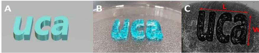
**Figure 14.** Evaluation of the printing accuracy. A: Theoretical model, B: Printed shape and C: measurement.
