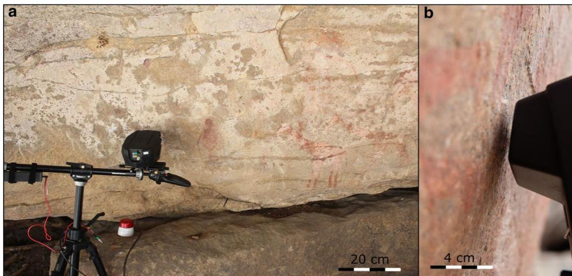
Fig. 2 The portable X-ray fluorescence ELIO spectrometer device during the analyses of Ghost Cave paintings (a) and Cycle of Life shelter (b)
